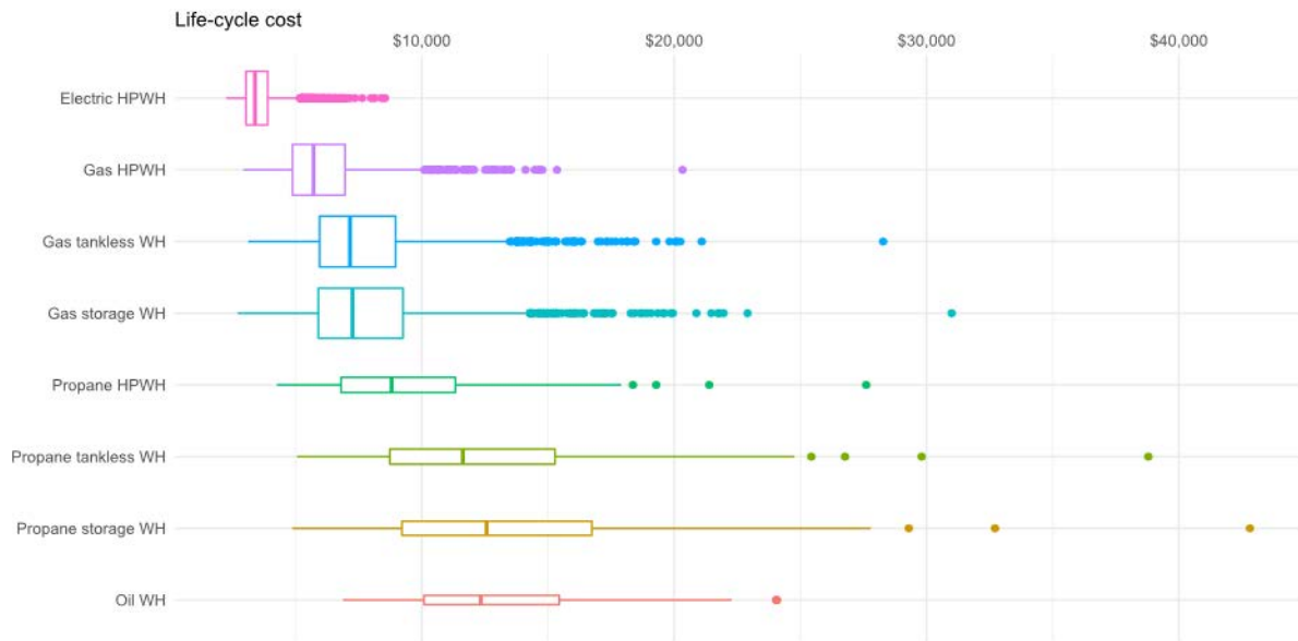
Figure 26. Life-cycle costs for water heating by system type. The lines in the middle of the boxes are the medians, the boxes show the upper and lower quartiles, the whiskers off the boxes show the most extreme data points within 1.5 times the length of the interquartile range, and the dots are individual outliers. Costs are in 2020$.
