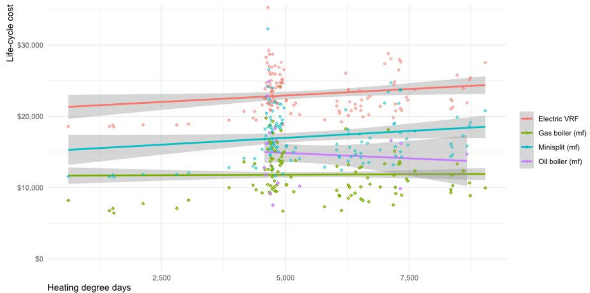
Figure 21. Life-cycle cost and best-fit lines for electric heat pumps (mini-split and VRF) and condensing gas boilers for apartments using low heat pump costs and medium energy costs in buildings with five or more units. Costs are in 2020$.
